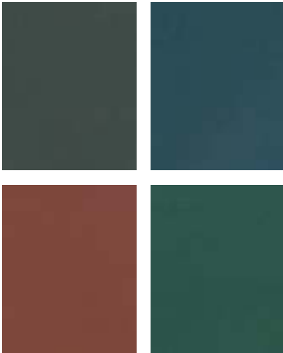
Figure 2. Kynar roof coatings using spectrally selective pigments from Ferro Corporation allow Classic Roofs to produce aluminum and steel shingles in several dark colors that meet Energy Star minimums with solar reflectances better than white asphalt shingles. Tests indicate that the colors will sharply reduce solar heat gain through the roof.
