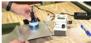
Measuring Thermal Emittance of Coating Tent Fabric
